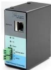
BMS Series of Converters are Building and Industrial Automation multi-protocol device server for OEMs wanting to provide protocol translation between Serial-Serial, Serial-Ethernet and Ethernet-Ethernet devices using LonWorks®, BACnet, Metasys N2, Modbus and more.
