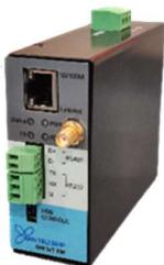
GW IoT EM is a gateway used for remote monitoring of multiple field equipment via Ethernet WAN and WiFi network. It acts as a Modbus master to multiple Modbus slave field devices at a single location on serial and provides reliable data connection to a web-based application server. The Web Server application can be hosted on public network or can be installed at central monitoring station having Static IP. It is designed to be used in industrial panels and operates on 9V-30V DC power supply.
