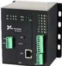
Sensors are used to continuously monitor and control various process parameters. These measurements help improving processes for adhering to product specifications & improve product quality. Monitoring and controlling Temperature, Pressure, Level, Flow etc are common occurrences for any process. IO Converters convert the Analog & Digital data from Sensors to Modbus to be taken to SCADA for further processing
