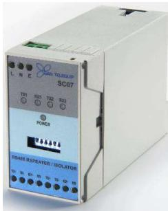
SC07 is used to expand Line driving capability of RS485 / RS422 beyond 1.2 km. It also converts RS485 to RS422 ( and vica versa ). It can also be used as RS485 Isolator. They are used for providing Isolation to Serial Interface. With high degree of protection, it keeps the COM port of your equipment safe.
