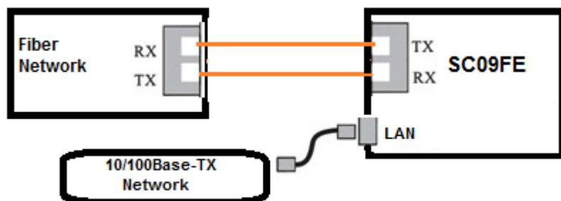
The network device (work station, hub or switch) with RJ-45 interface is connected to RJ-45 jack of optical transceiver through twisted-pair. The multi/single mode fiber is connected to the fiber interface of the optical transceiver then switch on etc. The corresponding LED is on for correct connection. (See the table below for the LED indicators)
