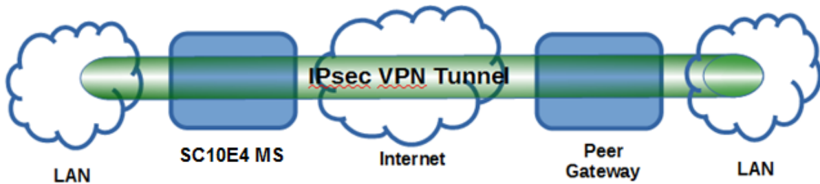
Figure 2.26 Example of network application using subnet-2-subnet connection via SC10E4 MS and a peer device
