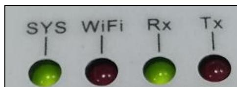
**SYS (Green)** : Power indicator. When the power is on, the LED will be on and blink per second.
